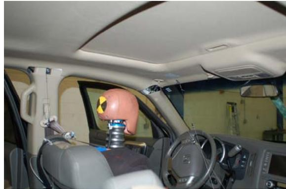
**Figure 5. String Potentiometers to A Pillar**
