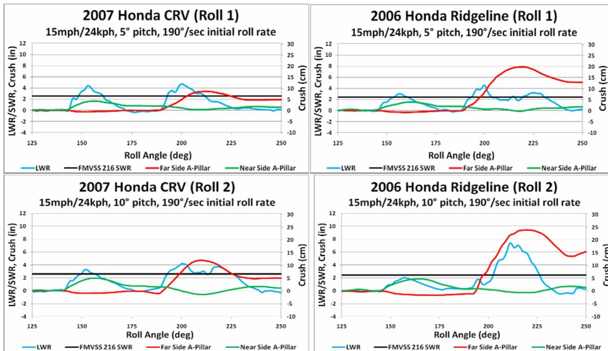
Figure 9. CRV Roof Crush vs. Roll Angle.
