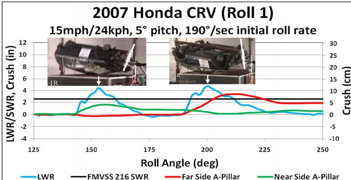
Figure 8. 2007 Honda CRV Test Results with Actual Vehicle Positions at Peaks.
