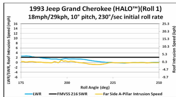
Figure 38. JGC w/HALO™ Roll 1 Intrusion Speed
