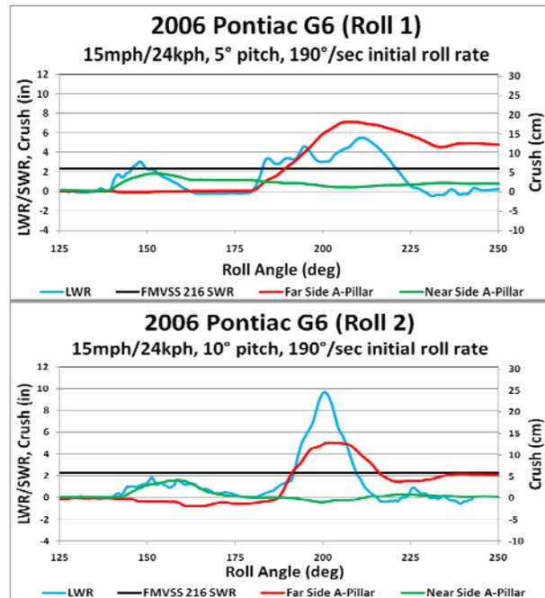
Figure 14. G6 Roof Crush vs. Roll Angle.
