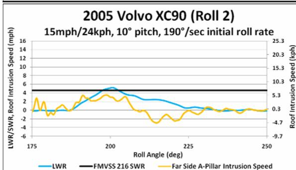
Figure 19. XC90 Peak Roof Intrusion Speed.
