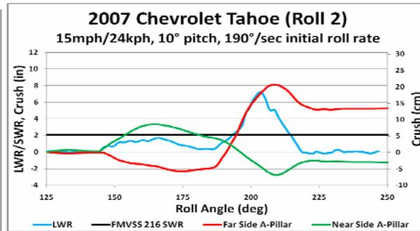
Figure 18. Tahoe Roof Crush vs. Roll Angle.
