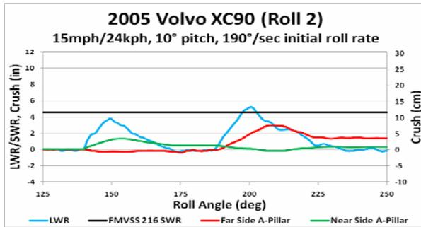
Figure 17. XC90 Roof Crush vs. Roll Angle.
