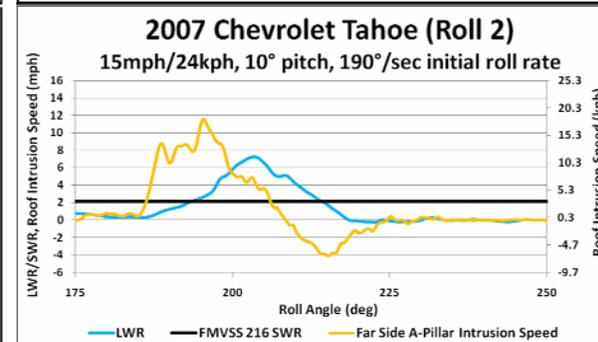
Figure 20. Tahoe Peak Roof Intrusion Speed.
