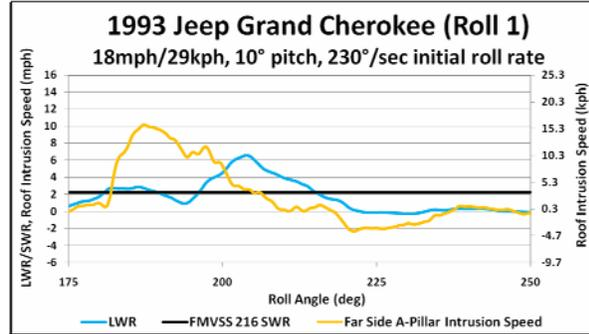
Figure 36. JGC Peak Roof Intrusion Speed.
