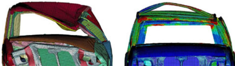
**Figure 32. FEA – Finite Element Analysis with HALO™, Before and After One Roll.**
