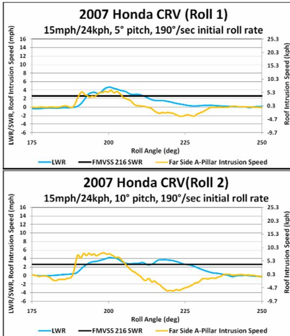
Figure 11. CRV Peak Roof Intrusion Speed.
