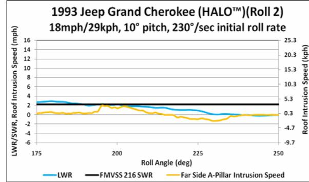
Figure 40. JGC w/HALO™ Roll 2 Intrusion Speed
