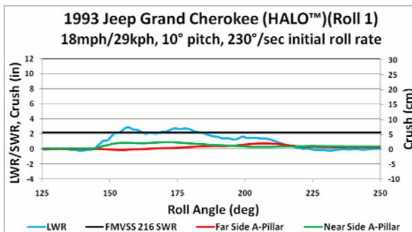
Figure 37. JGC w/HALO™ Roll 1 Roof Crush
