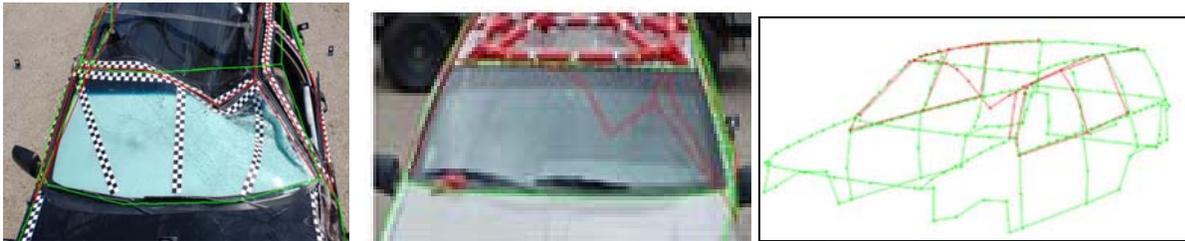
**Figure 29. 1993 JGC's JRS Rollover Tested With and Without HALO™ and the Corresponding Photogrammetric 3D Analysis.**
