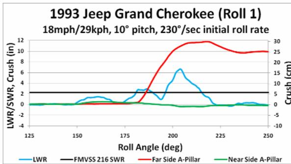
Figure 35. JGC Roof Crush vs. Roll Angle.
