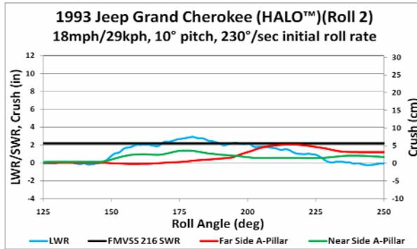
Figure 39. JGC w/HALO™ Roll 2 Roof Crush
