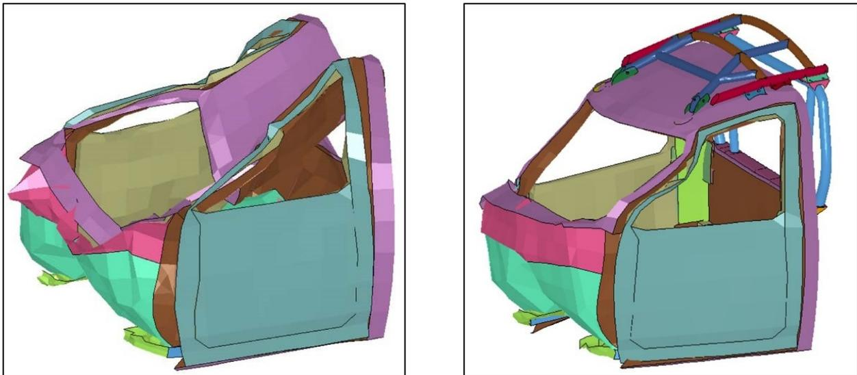
Figure 12. Comparison of intrusion over driver seat position
